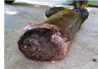
EXTERNAL SHORT CIRCUIT
