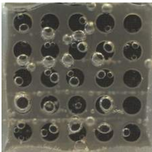
DMFC4. Passive DMFC under high current density.
